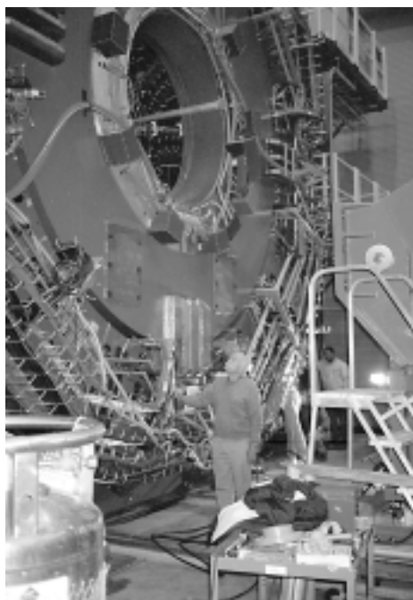
Fr. Tom McShane, S.J., is dwarfed by the STAR time projection chamber of the RHIC experiment.
